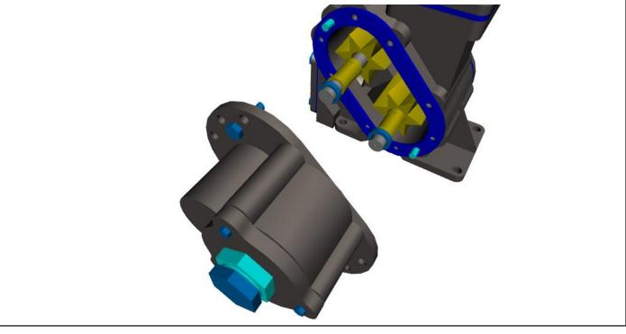
Install the Bolts on the Face Plate Assembly, Relief Valve.
